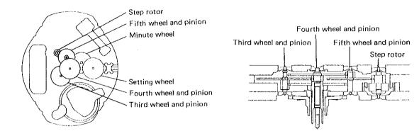
Note: Set the step rotor with its pinion facing toward the main plate side.
