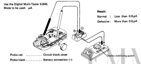
Set the display stabilizing switch of the tester to the "B" position.
