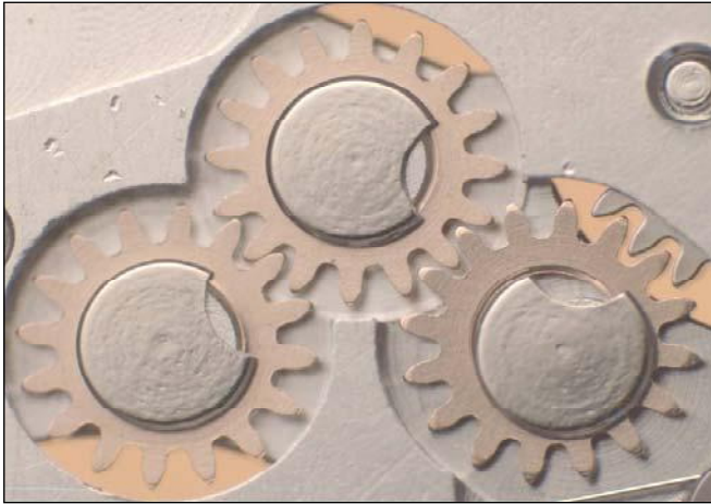
Lubrication of the 3 intermediate driving wheels for ratchet wheel (HP 1300 Sans Colorant)
